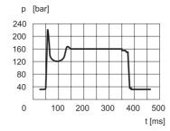
Diagram noted passing from maximum flow rate to zero flow rate and vice versa
